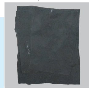
MWNT/SBR Composite Film made by Banbury mixer The bad dispersion of CNT shows the gray color and surface irregularity of the film.
