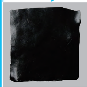
MWNT/SBR Composite Film made by ARE-310 The uniform dispersion of CNT shows the dark black color and smoothness of the film.
